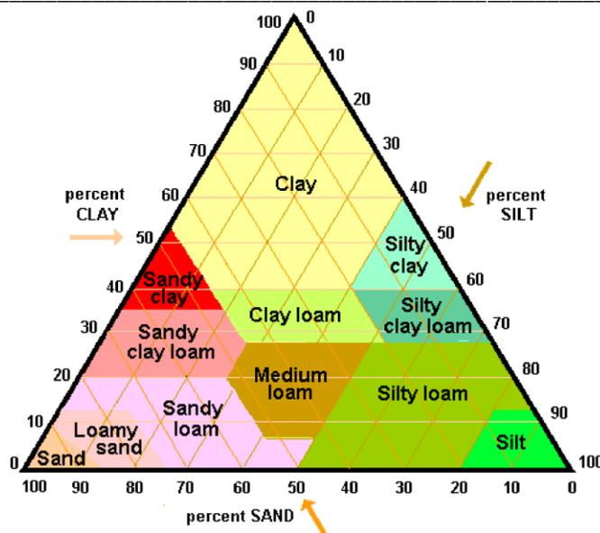
Figure 2. USDA textural triangle for demonstration of soil texture
